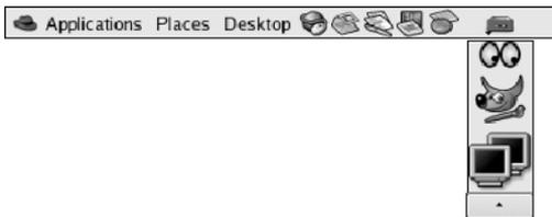
**Figure 3-10:** Add launchers or applets to a drawer on your GNOME panel.
