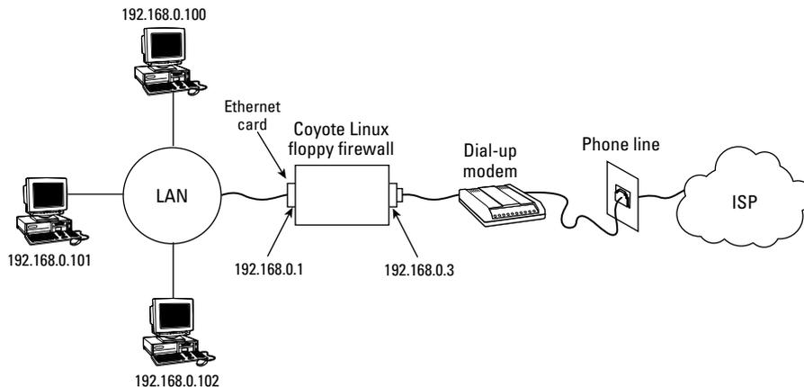
**Figure 18-2:** A Coyote Linux firewall runs from a floppy disk, managing traffic between your network and the Internet.
