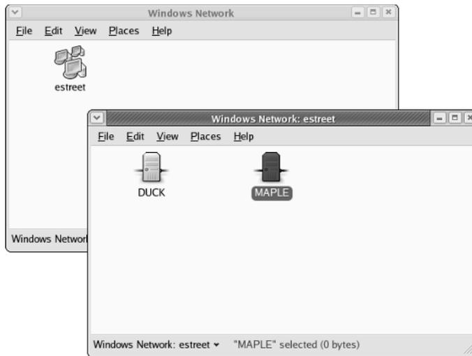
**Figure 3-12:** Display shared Windows file and printer servers (SMB) in Nautilus.
