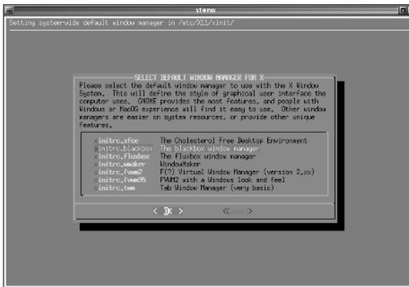
**Figure 3-15:** In Slackware, you can change window managers using the `xwmconfig` command.
