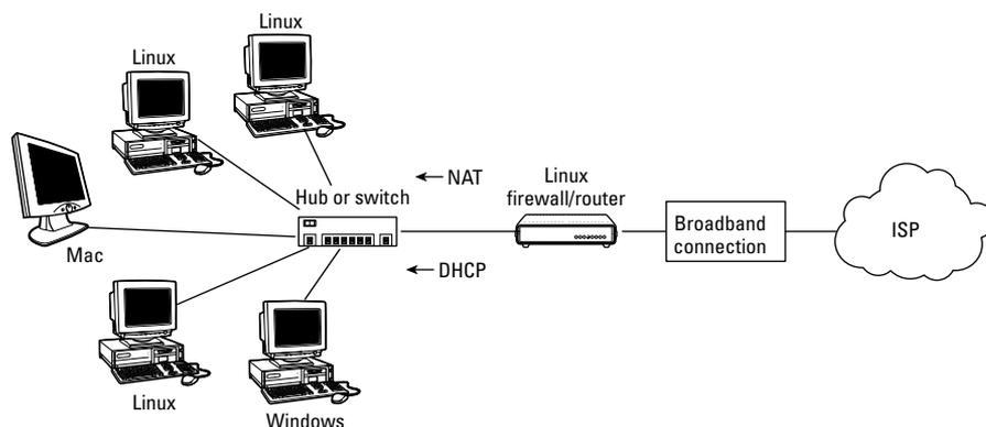
**Figure 5-3:** A firewall provides a safeguard between your LAN and the Internet.
