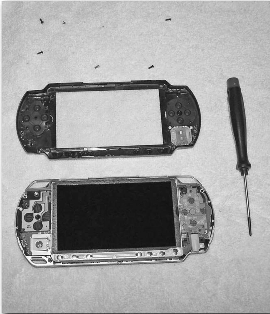
FIGURE 4-6: The first layer of PSP guts
