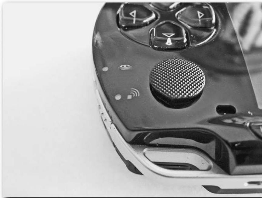
FIGURE 5-1: The wireless access light on the PSP
