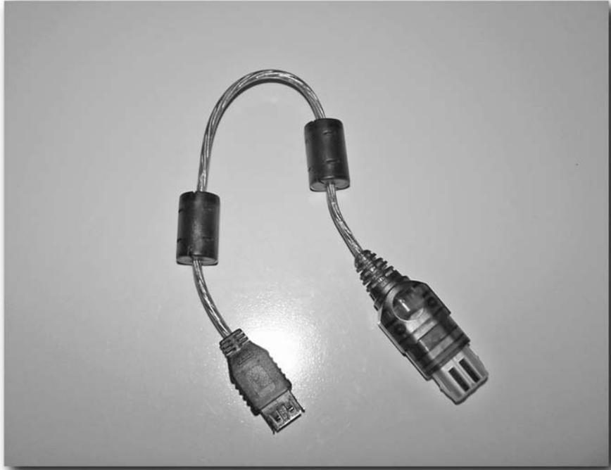
FIGURE 3-15: The Xbox Controller USB Adapter
