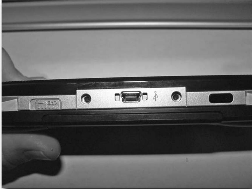
FIGURE 3-13: The USB port on the PSP
