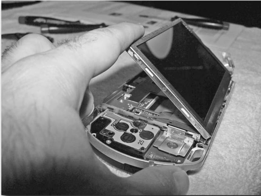
FIGURE 4-9: The screen partially removed
