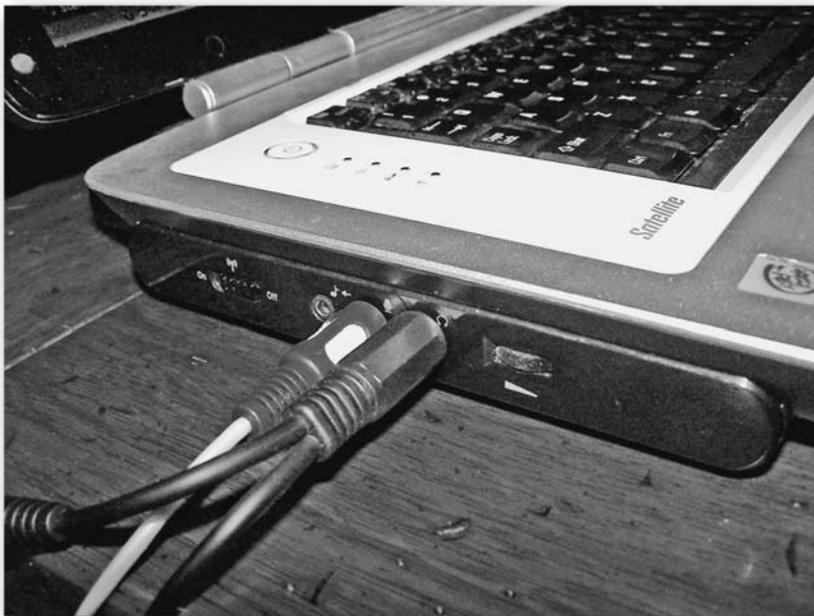
FIGURE 11-4: The audio cable properly connected
