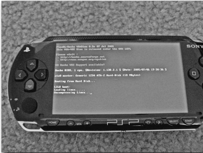
FIGURE 15-2: Bochs loading Linux on the PSP
