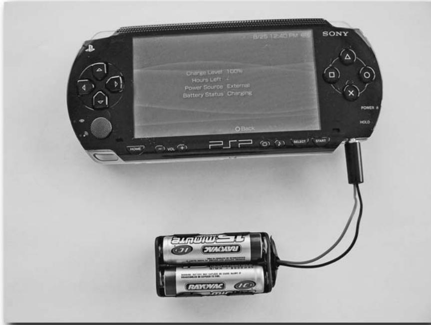
FIGURE 13-12: The external battery pack in action
