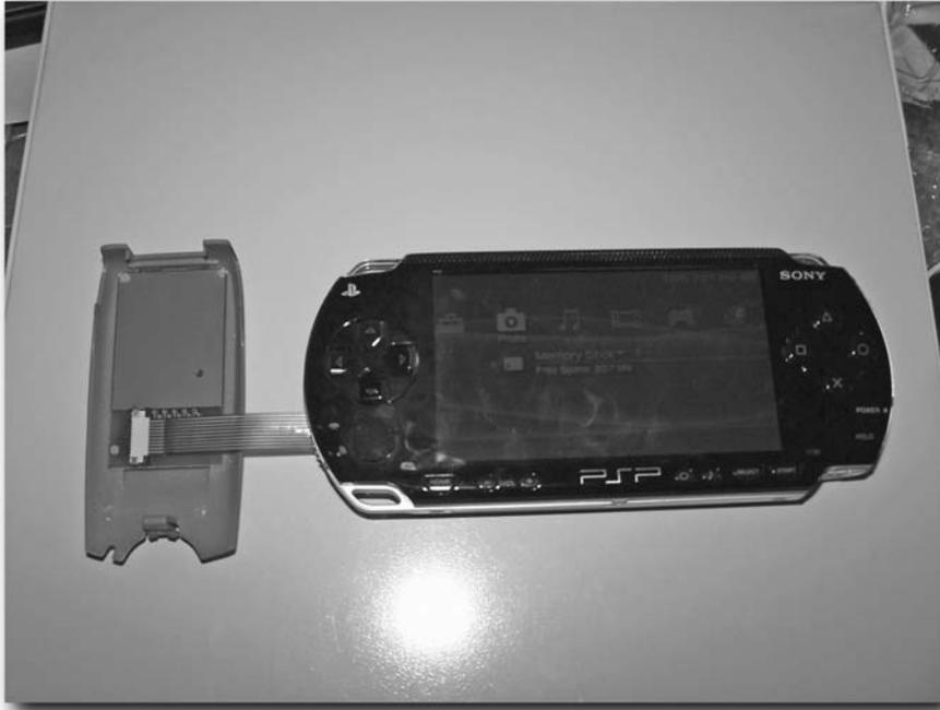
FIGURE 3-3: The adapter in the PSP's Memory Stick Duo slot
