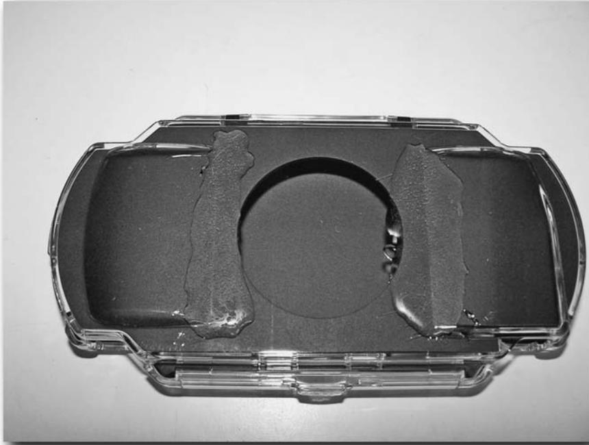
FIGURE 14-19: Applying the epoxy
