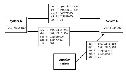
The host machine will receive the spoofed packet with the correct acknowledgment number and will have no reason to believe it didn't come from the victim machine.
