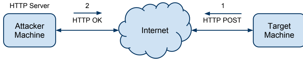
Figure 3.3: Exfiltration using an HTTP POST action
