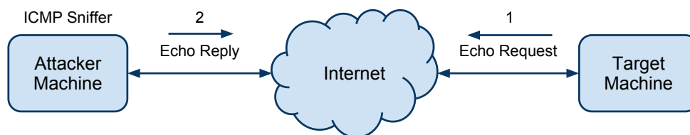
Figure 3.8: Exfiltration using ICMP Echo Request packets
