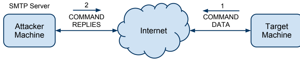
Figure 3.5: Exfiltration using an SMTP server
